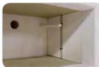
Thermocouple in furnace chamber and ventilation chimney
