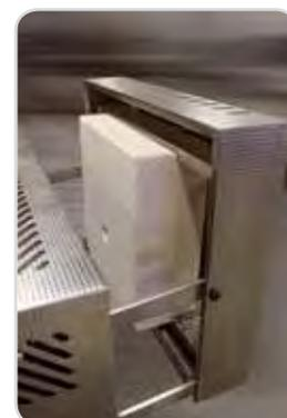
The door insulation with the peephole for batch control
