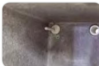
Thermocouple and ventilation chimney in the furnace chamber
