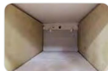
Furnace chamber with thermocouple and ventilation chimney
