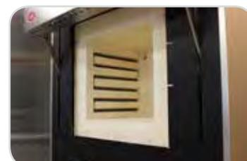
Heating coils in grooves built into the lining
