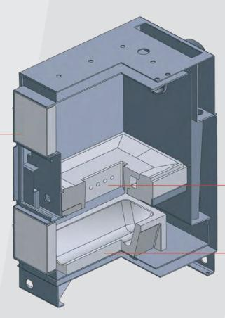
Shaped blocks for stoking chambers
