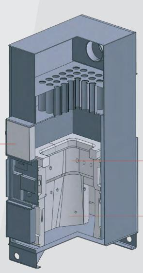
Shaped blocks for secondary combustion chambers
