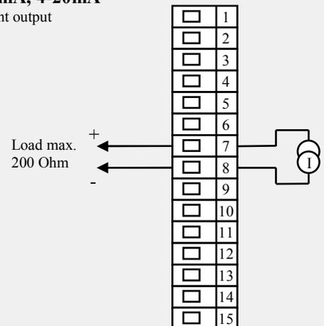
Current output *is galvanically isolated* from the device's ground
