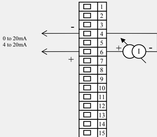
Retransmit output is galvanically isolated from the device's ground
