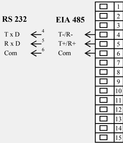
Communication line is galvanically isolated from the device's ground
