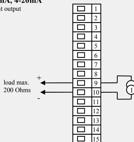
Current output is *isolated* from the device's ground
