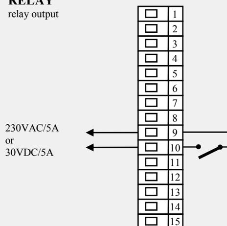
RELAY output is *galvanically isolated* from the ground of the controller. For this output it is necessary to fix the wires in the way that in case of loosening the wire from the terminal the insulation would not be reduced between supply voltage and safety voltage.
