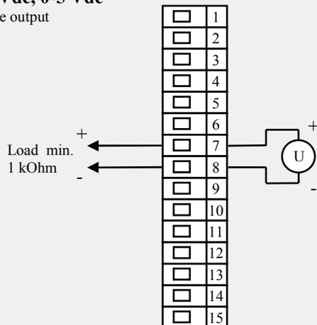
Voltage output *is galvanically isolated* from the ground of device
