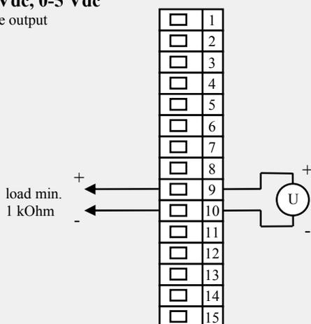
Voltage output is *galvanically isolated* from device ground
