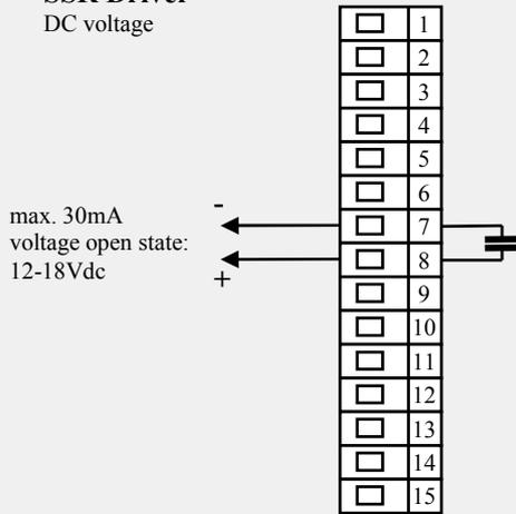
Output for ssr *is not isolated* from the ground of device
