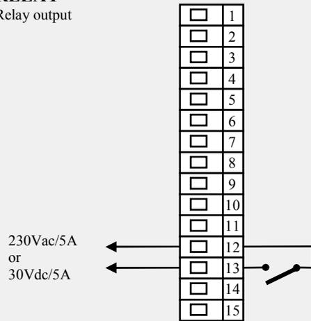
**RELAY output is *galvanically isolated* from the ground of the controller. For this output it is necessary to fix the wires in the way that in case of loosening the wire from the terminal the insulation would not be reduced between supply voltage and safety voltage.**
