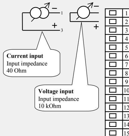
Measuring input is not galvanically isolated from the ground of controller
