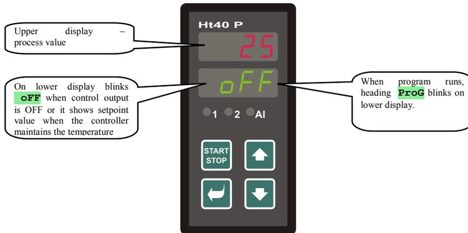
Upper display shows process value, Lower display shows **oFF** when the output is switched OFF or it shows set point value.
