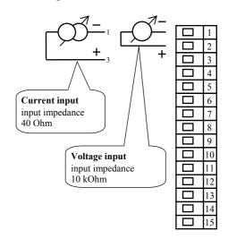
Measuring input is not isolated from the ground of controller
