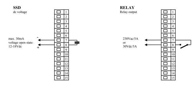
SSD is not isolated from controllers ground
