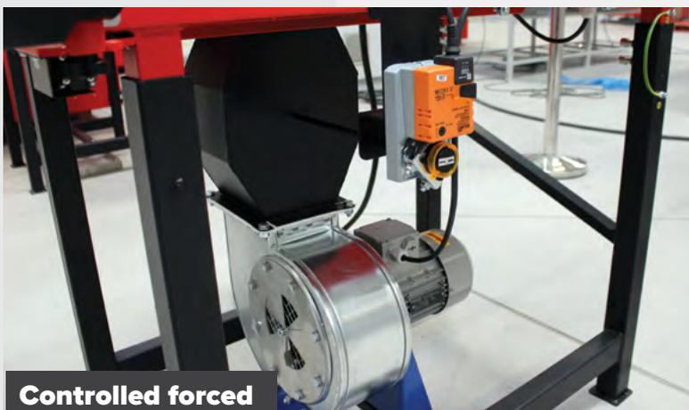
**Controlled forced pressure cooling**
