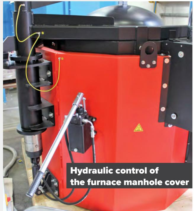
**Hydraulic control of the furnace manhole cover**
