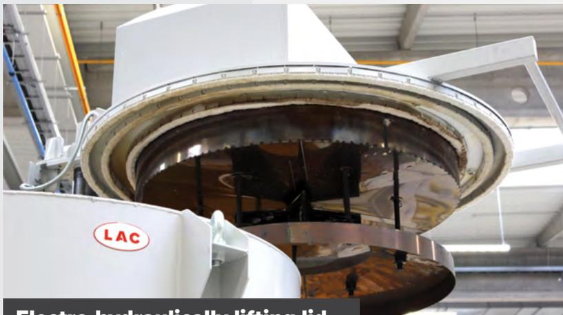
**Electro-hydraulically lifting lid**
