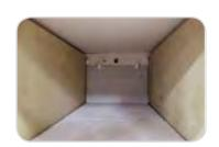
Furnace chamber with thermocouple and ventilation chimney
